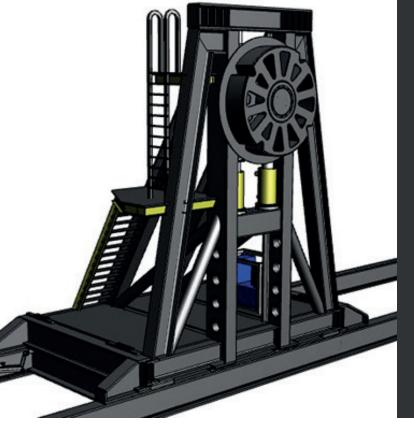
The system comes with a hydraulic power pack and a wireless control unit. The complete RDS system, including power pack and accessories can be transported by road in 20 & 40 foot containers. Each system comes with certified rigging and suitable cables and hoses. Skidding beams and skidding hydraulics are optional, while one can use the same powerpack that drives the RDS for skidding the towers.
